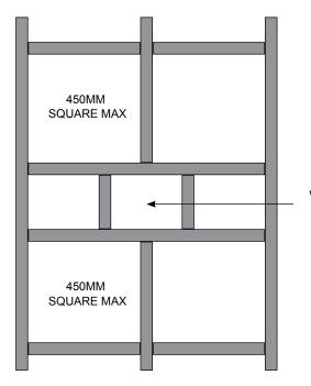
450mm centres on joists to be trimmed out. Tile Tray can span no greater than 450 x 450. Failure to follow floor detail will void warranty. Floor joists and trimmers must be flat, planning or sanding off any ridges is recommended before installation. Trim edges of base to support join of flooring and Tile Tray.
